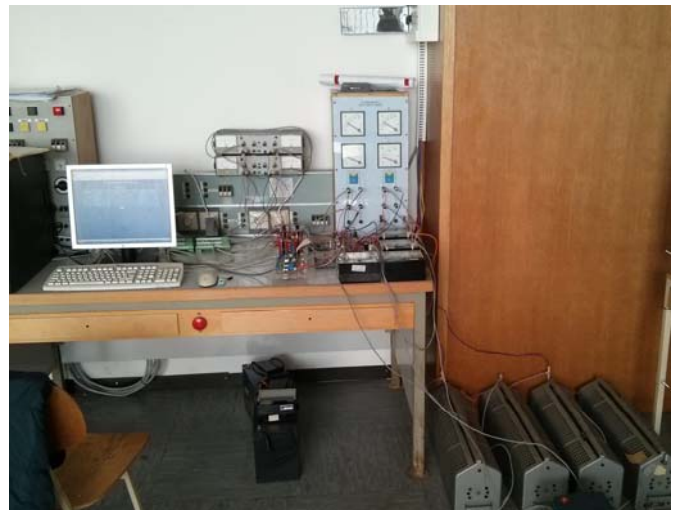
Figure 2. Test equipment with measuring instruments and MPPT converter
