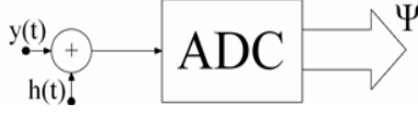
Figure 1. Block diagram of application of a uniform random dither h to the measured signal y .
