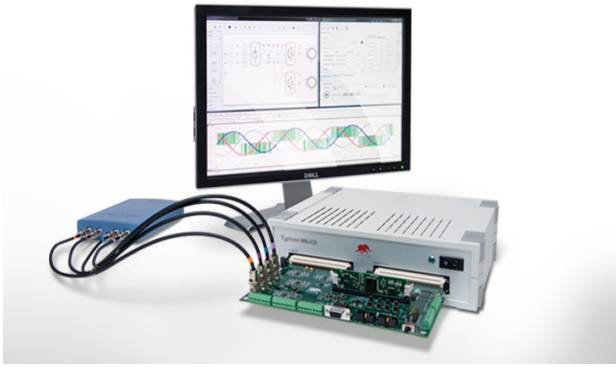
Figure 1. Educational setup with DSP controller and HIL
